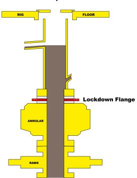
The Lockdown System is easily installed on many different sizes and types of bell nipple systems. Once installed, the Lockdown Flange replaces and functions as the rig's bell nipple flange. The Lockdown Lubricator System is utilized by land and barge rigs, jackup rigs, deepwater TLP and spar platforms globally.
