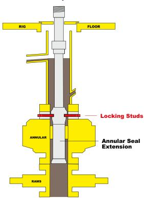
When logging operations are to be performed, WCS' lubricator is simply lowered through the rotary/bell nipple until properly located. The locking studs on the Lockdown Flange are engaged, anchoring the lubricator to the rig's BOP. The rig's annular BOP is then sealed around the Lockdown Lubricator's annular seal extension.
